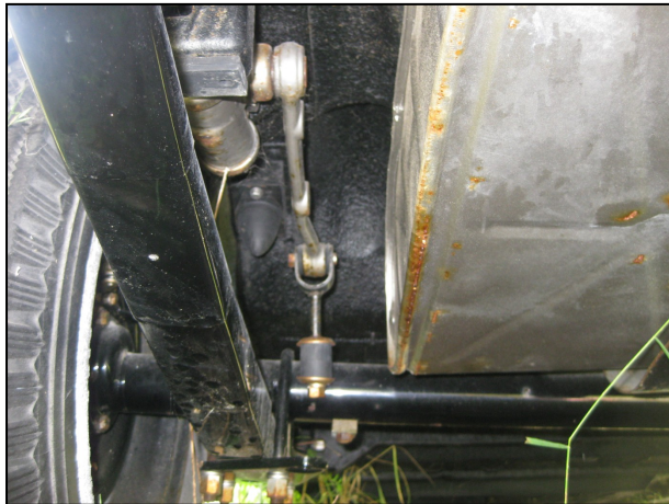
Shocks and gas tank. The springs were repainted. The fastenings rusting.
