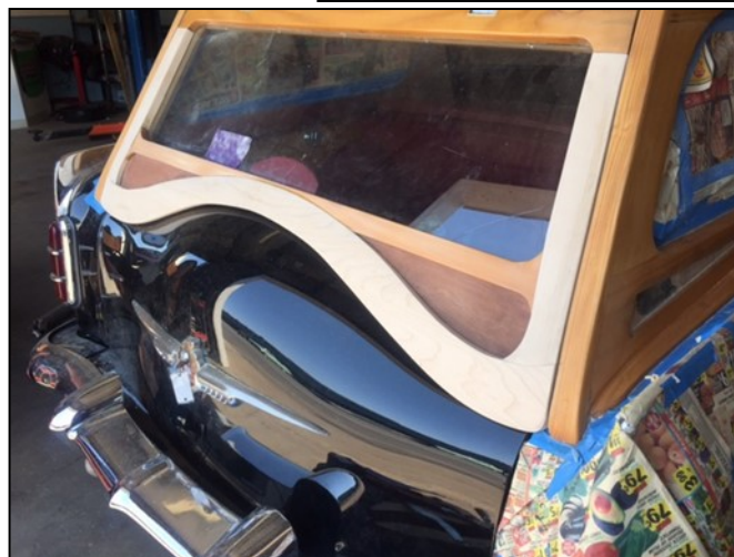
Tailgate - Damaged wood removed, new wood fitted, and stained
