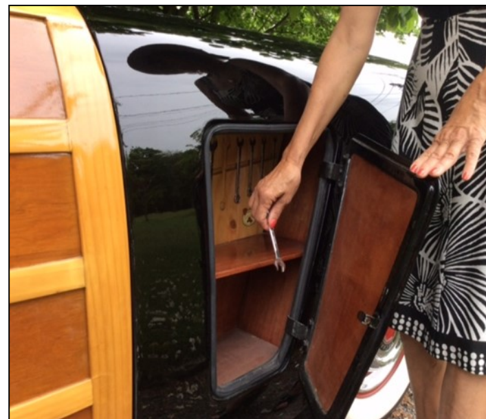
Custom European-style tool compartment in fender
