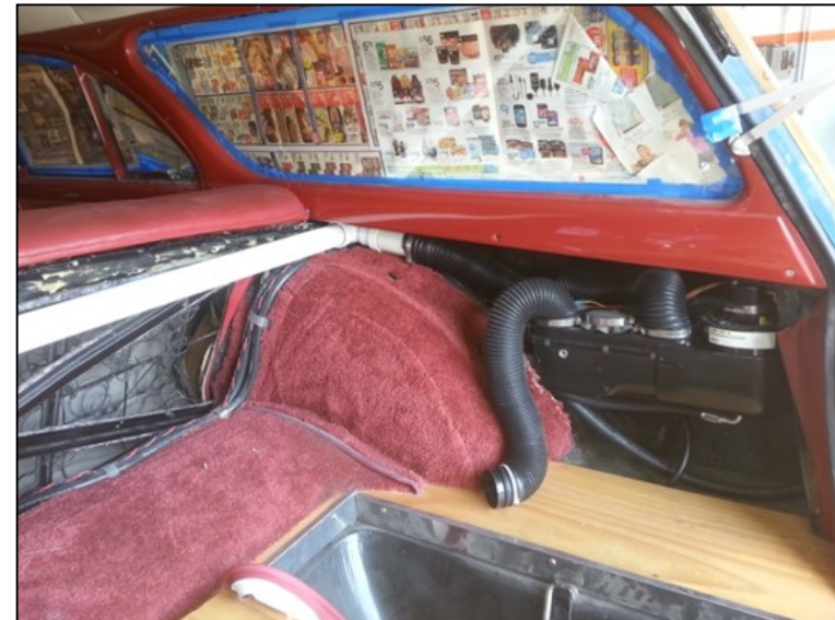
Ductwork and ac unit in cargo area
