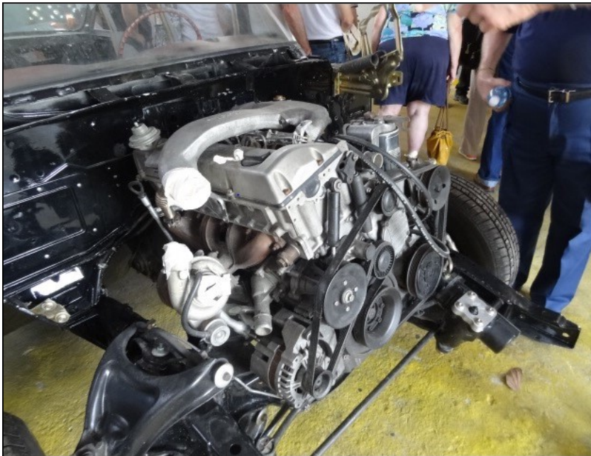
1959 Chevy with Mercedes Diesel engine under restoration.
